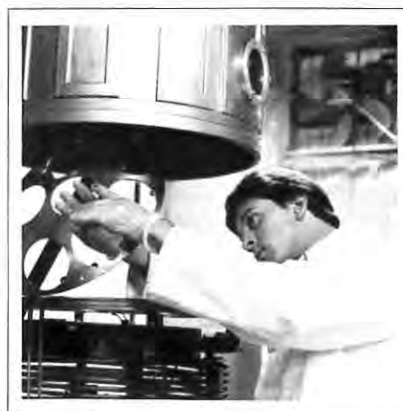
Fig. 2: Loading chrome blanks prior to vacuum deposition.
