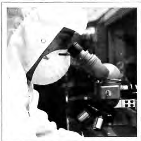
Fig. 1: Inspecting TFEL lamps under a binocular microscope in the clean room.
